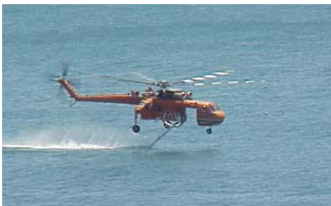
Sky crane taking on water from the Pacific Ocean. Drafting 2,800 gallons of water would take approximately 30 seconds.
